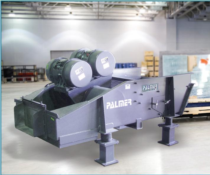
This unit not only acts as a shakeout deck, but also includes an integral attrition mill section. The output of this unit is grain size and ready for cooling and classification. The low level deck offers ease of loading with a forklift, roller conveyor, or vibratory feed conveyor. No pit is required which means less cleanup and failed springs from being buried.
