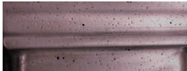
*Pin Hole Porosity on outer surface of Casting. This was caused by a reaction between the molten aluminum and mold coating.*
