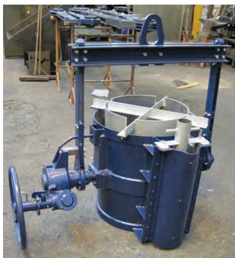
As the teapot shape provides a good anchor for the castable refractory, wrecking out the lining is likely to be labor intensive and require the use of pneumatic hammers etc., all of which creates health and safety issues.
