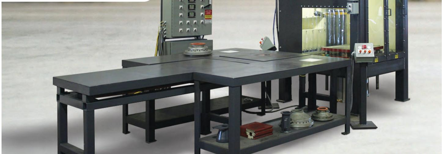
To begin core making, the RFID interrogator built into the core maker bench, reads the tag's number, and transmits that information to the PLC. Then, the computer retrieves the settings for that core. The worker presses one more button to begin the core making process, and the core box is moved into the core blower. The computer instructs the blower accordingly and injects sand and chemicals before purging the box.
