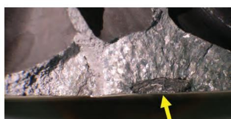
*Magnesium Oxide Inclusion on the failure surface of this part.*
