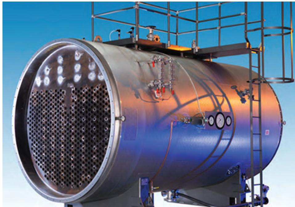
recovery process is to move the wasted heat from the hot and dirty exhaust gas stream into some useful process; such as making your own electricity. If you can manage that you will effectively reduce your carbon footprint in some cases by almost 50%.
