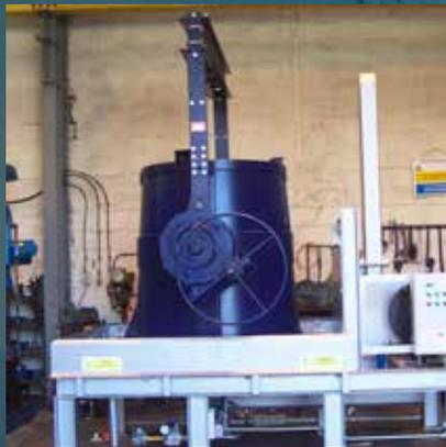
*Acetarc ladle pre-heater with Acetarc ladle*
