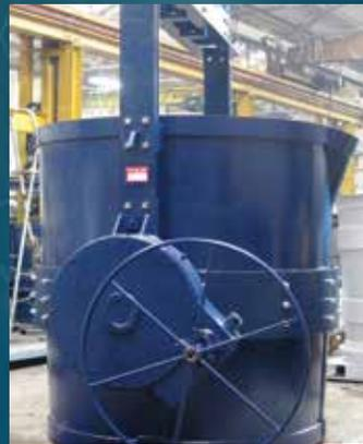
*Acetarc 15t capacity heavy-duty ladle*
