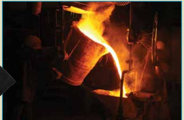
Powered rotation, using either electric or pneumatic motor drive units, is a standard option. Other tilting options, such as using hydraulic rams, are also available.
