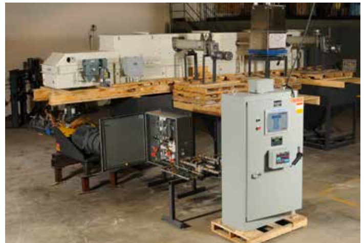
Aggregate mixing system with weigh-belt feeder
