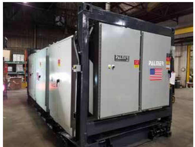
Triple mass flow pumping system (skid mounted)
