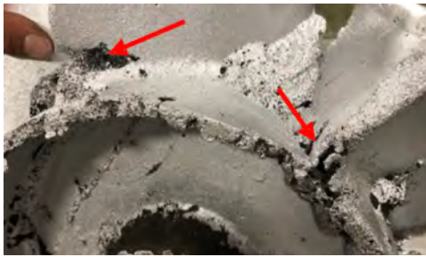
Residual sand and dross on scrap castings should be removed prior to placing in the furnace.
