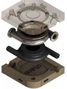
This digital rendering shows a cope, drag and core that was 3D printed on the Viridis3D RAM 123.
