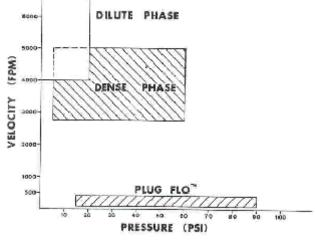
Fig.1 Types of Pneumatic Conveying Systems
