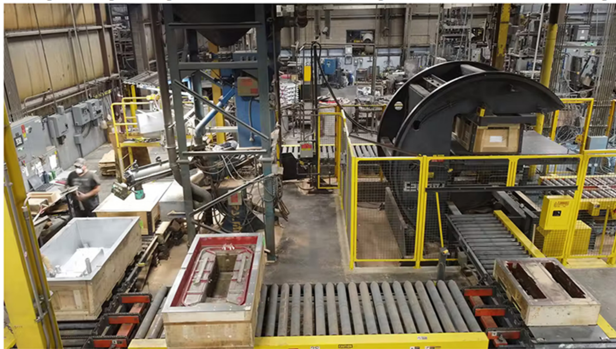
To increase Eck Industries’ casting throughput while reducing manual labor, Palmer Manufacturing custom-designed a new C-frame rollover molding machine.
