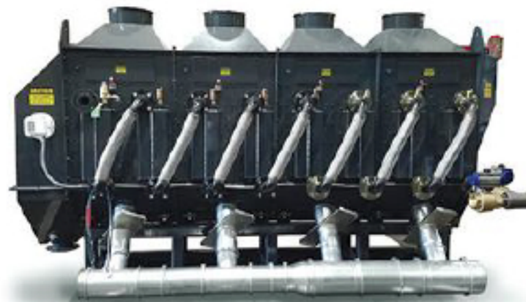
Palmer Manufacturing's HCCL-Series sand classifier system has four major components: a base, or plenum chamber, into which fluidizing air is supplied by a blower; a fluidizing deck; a heat exchanger bundle; and a main body, which serves as a cover and pressure chamber.
