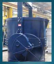
Acetarc 15t capacity heavy-duty ladle
